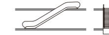
Single Escalator Use single escalator to connect two levels, it is suitable for buildings that Visitors flowrate mainly in one direction, flexible adjustments can be made to meet passenger flow needs.(for example: Up in the morning and down at night) .
